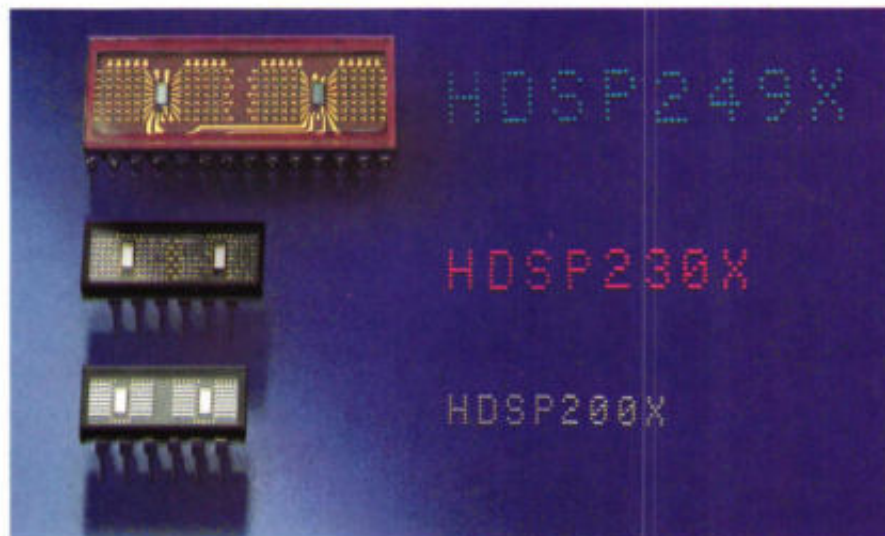
HDSP-2000 series, Characters show actual size HDSP-200X (3.8 mm), HDSP-230X (5.0 mm), HDSP-249X (6.9 mm)
